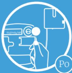
Connect the Smile P0 to the meter by connecting the round head of the cable on to the optical port of the main meter. Ensure that the P0 head is placed in such a way that the wire hangs straight down.
